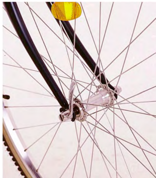
Figure 7 Quick Release Incorrect Position—Example 2
