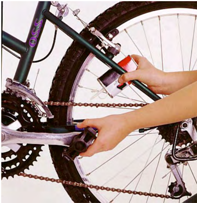
Figure 5 Lubricating the Chain
