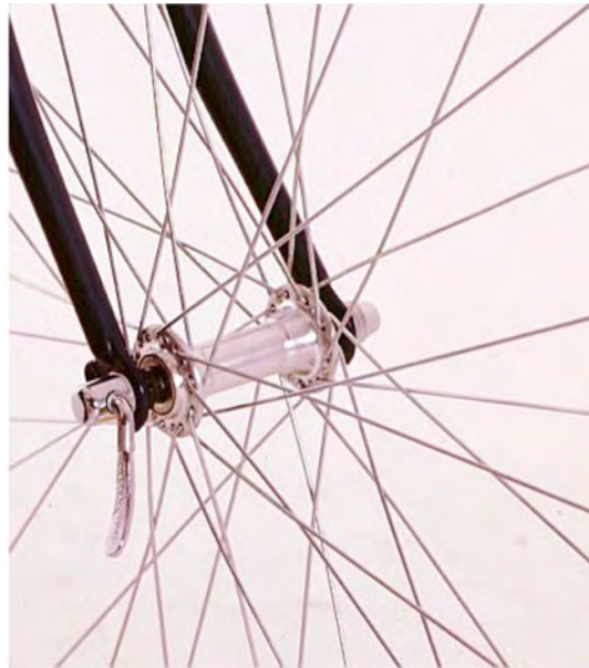
Figure 6 Quick Release Incorrect Position—Example 1
