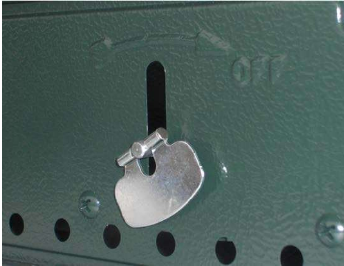
Figure 7 Auxiliary Burner Control
