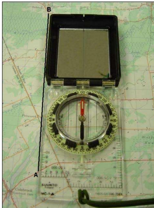
Figure 2 Measuring a Magnetic Bearing on a Map D Cds 3, 2007, Ottawa, ON: Department of National Defence
